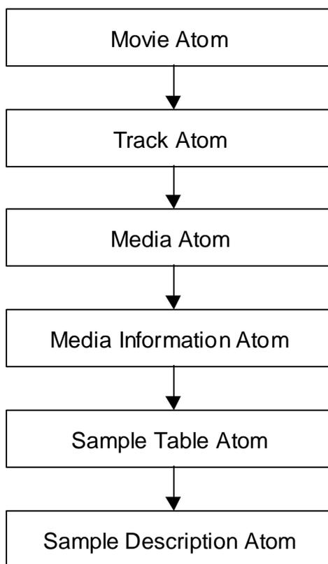
**Figure D.1: MP4 Atom Structure Hierarchy**
