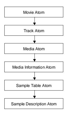
Figure D.1: MP4 Atom Structure Hierarchy
