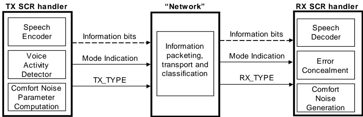
Figure 1: Block diagram of one link SCR operation
