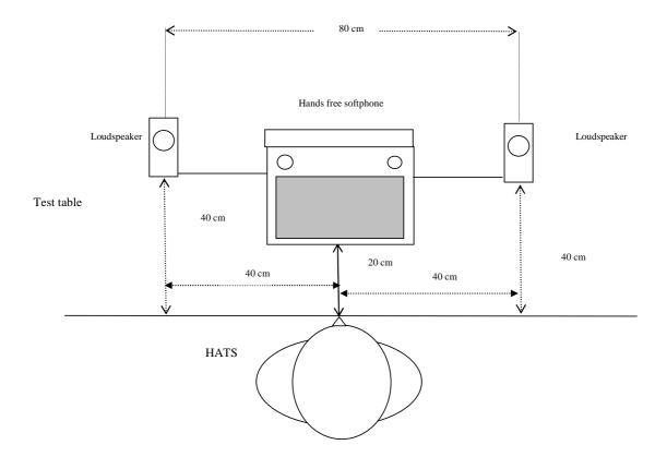
Figure 13: Configuration of a softphone using external speakers relative to the HATS viewed from above
