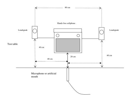
Where separate loudspeakers are used, the system will be positioned as in figure 12 or figure 13.
