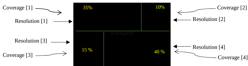
Figure D.1-3: An example of a viewport covered by four different quality ranking 2D regions
