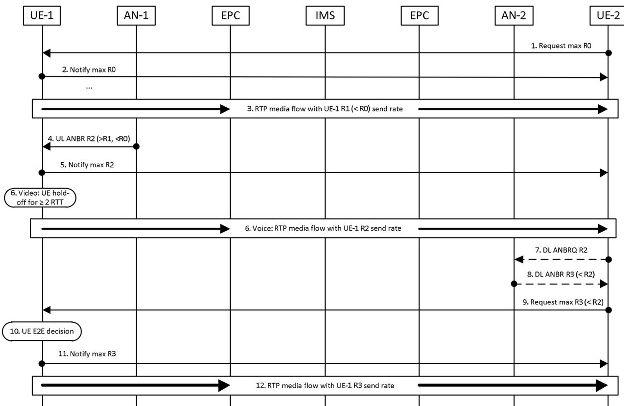
Figure 10.7-2 Uplink bitrate increase based on ANBR
