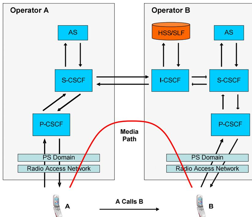
**Figure 4.1: High-level architecture figure showing two MTSI clients in terminals using 3GPP access involved in an MTSI call set-up. The terminals connect to the IMS network over a 3GPP radio access network.**
