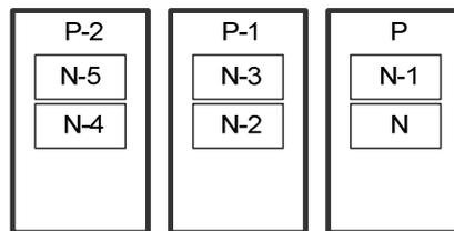
Figure 10.11: Payload packetization with 2 frames aggregated per packet
