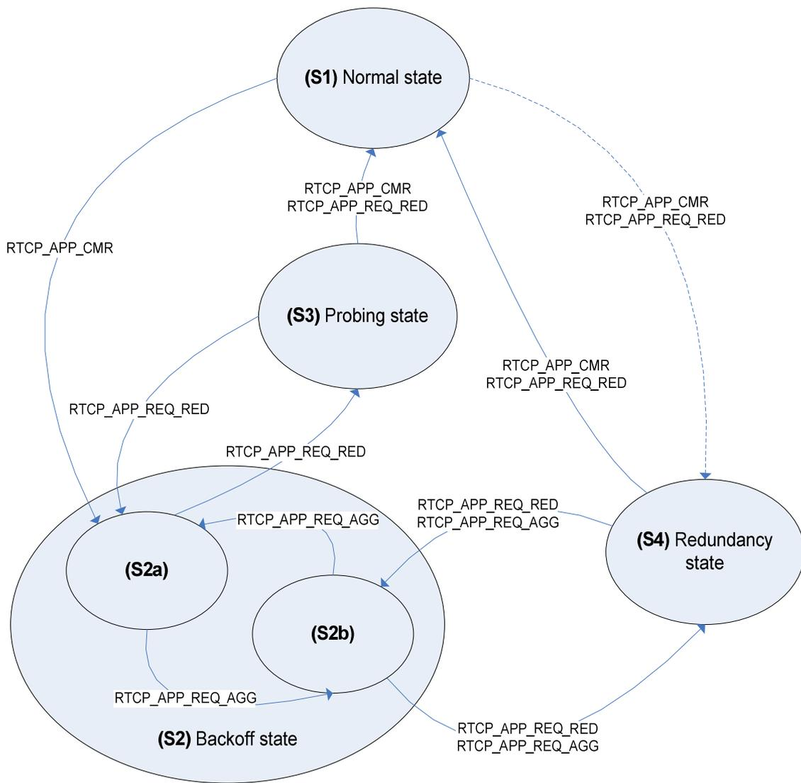
Figure C.2: State diagram for four-state adaptation state machine
