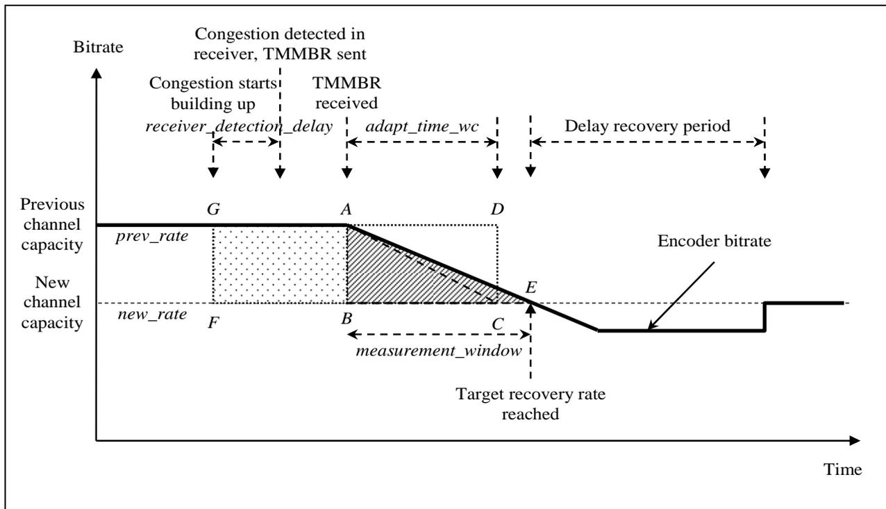
**Figure C.8. Schematic figure of bitrate reduction in video encoder when the encoder cannot immediately switch to the requested bitrate**
