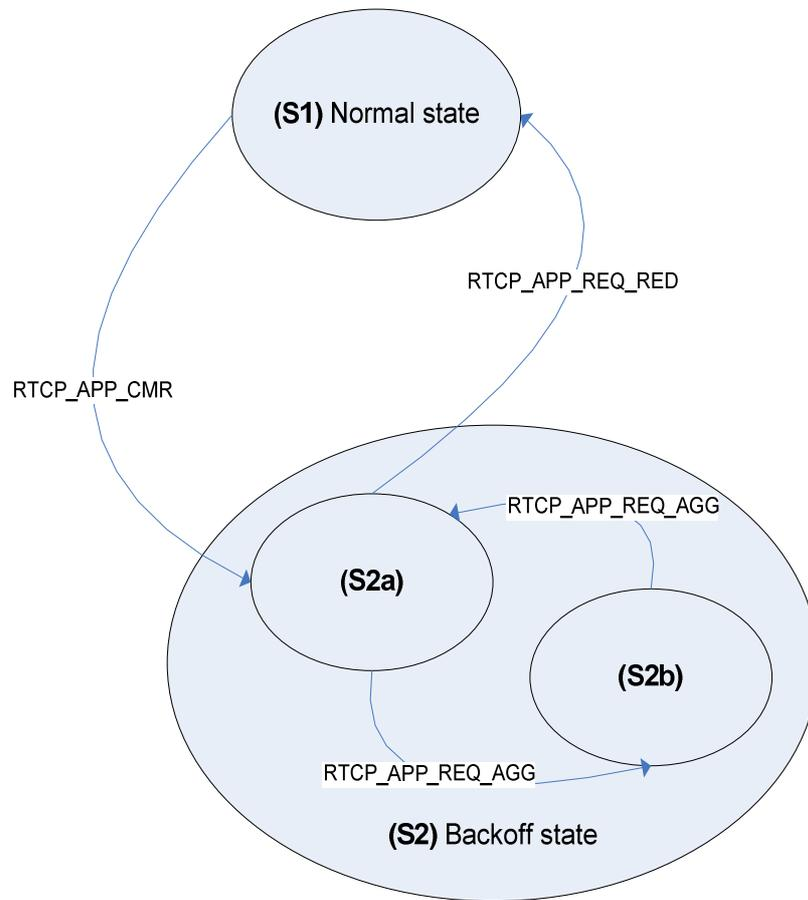
**Figure C.4: State diagram for two-state adaptation state machine**
