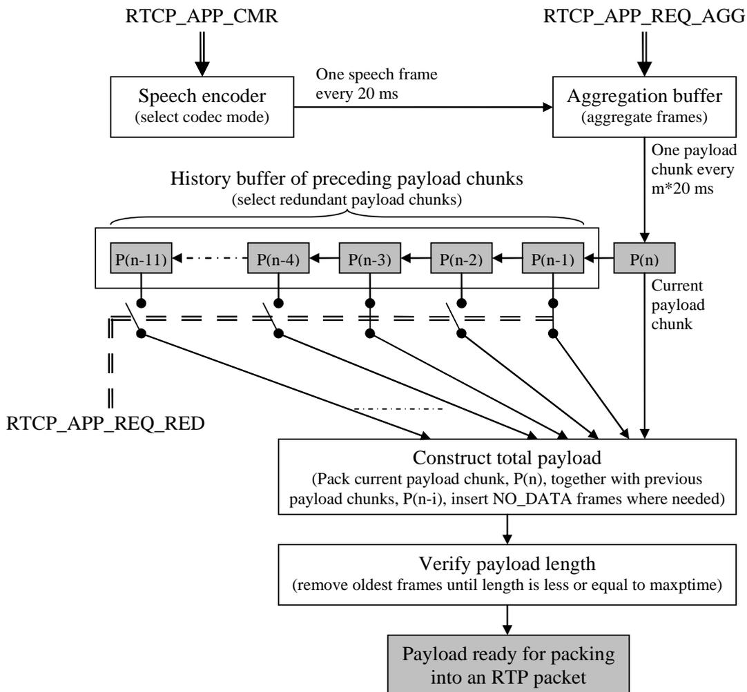
**Figure 10.6: Visualization of how the different adaptation requests affect the encoding and the payload packetization**
