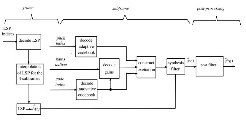
Figure 4: Simplified block diagram of the adaptive multi-rate decoder
