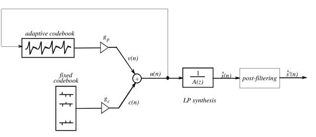
Figure 2: Simplified block diagram of the CELP synthesis model
