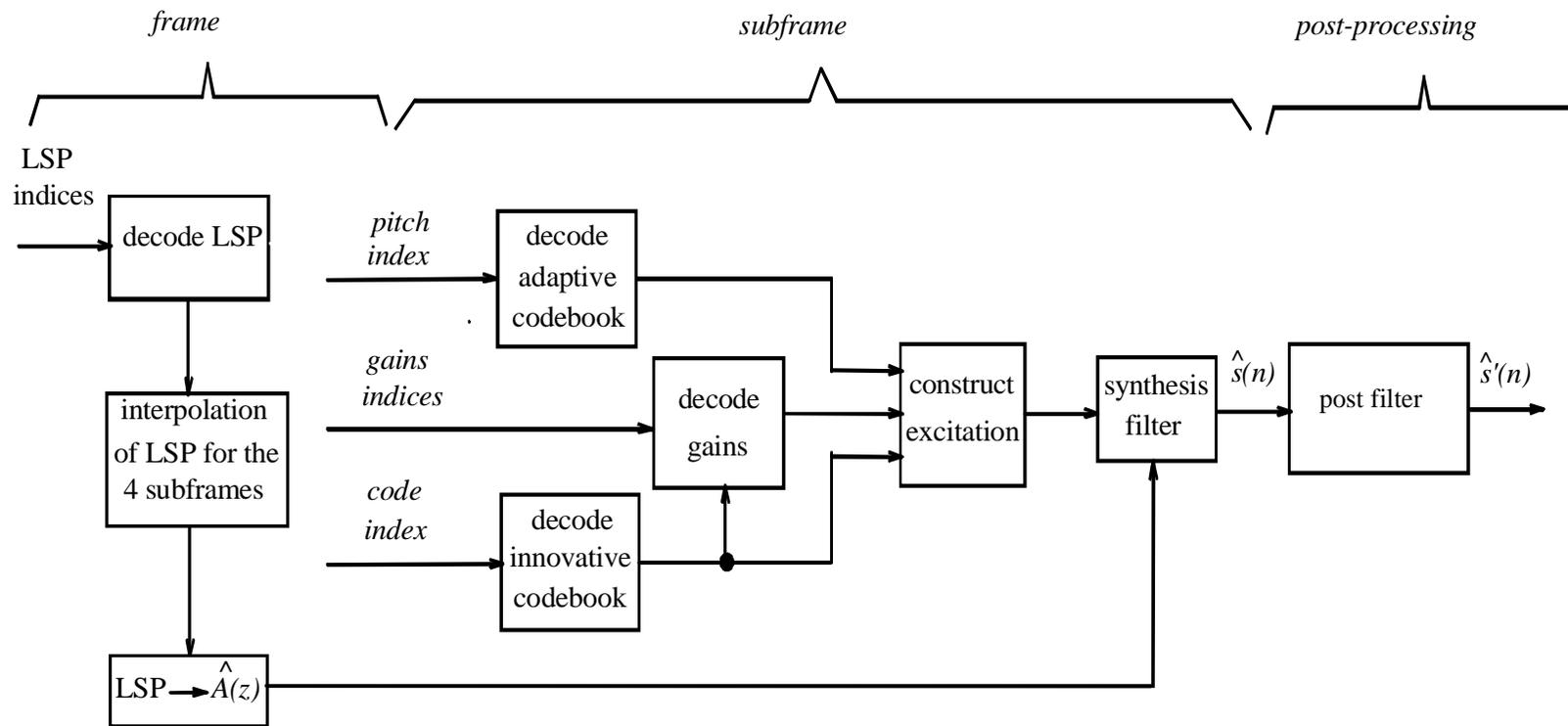
Figure 4: Simplified block diagram of the adaptive multi-rate decoder
