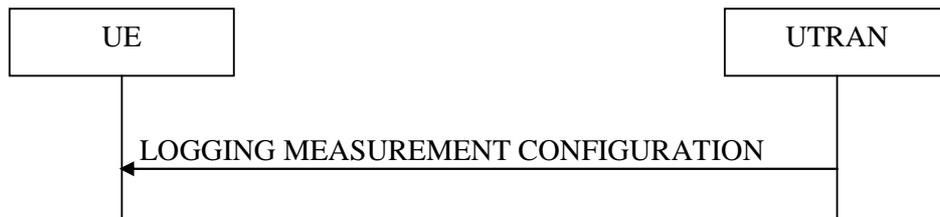
**Figure 5.3-1: ANR Logging configuration with Logging measurement configuration message**
