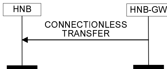
Figure 8.6.2.3.1: Connectionless Transfer procedure – HNB-GW originated – Iurh connection via the HNB-GW
