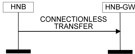
Figure 8.6.2.2.1: Connectionless Transfer procedure – HNB originated – Iurh connection via the HNB-GW.
