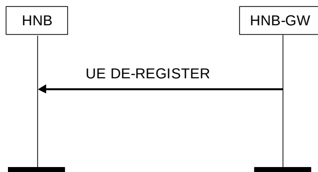
Figure 8.5.3-1: UE De-Register Procedure: HNB-GW Originated Successful Operation
