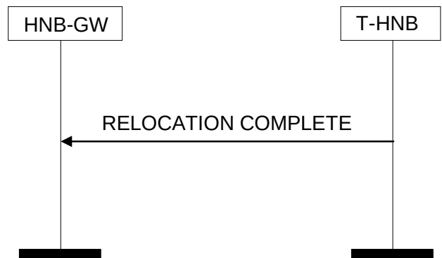
Figure 8.11.2-1: Relocation Complete procedure. Successful operation.
