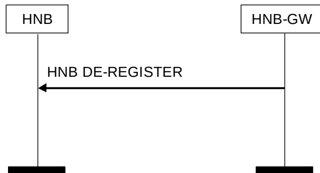
Figure 8.3.2-1: HNB De-register Procedure: Successful Operation
