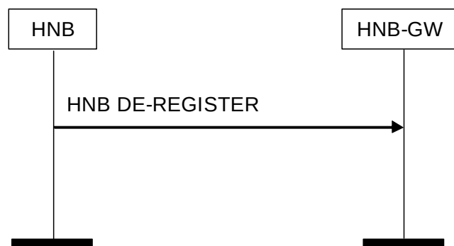
Figure 8.3.1-1: HNB De-register Procedure: Successful Operation
