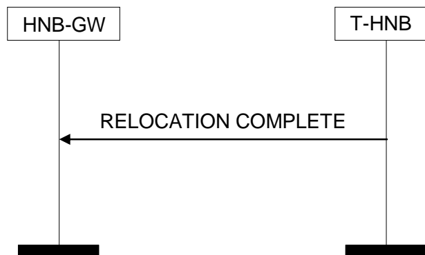
Figure 8.11.2-1: Relocation Complete procedure. Successful operation.
