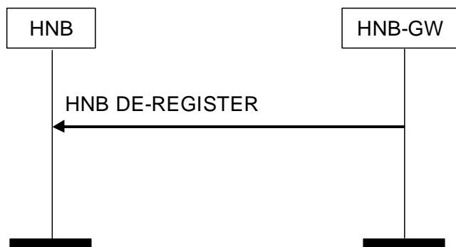
Figure 4: HNB De-register Procedure: Successful Operation
