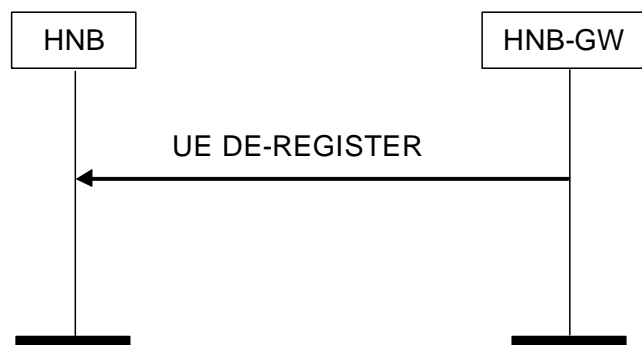
Figure 8 UE De-Register Procedure: HNB-GW Originated Successful Operation
