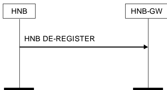
Figure 3: HNB De-register Procedure: Successful Operation
