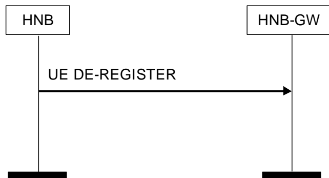
Figure 7 UE De-Register Procedure: HNB Originated Successful Operation
