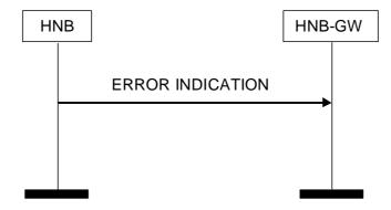
Figure 8 Error Indication HNB Originated, Successful Operation
