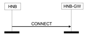
Figure 1: Connect to HNB-GW procedure
