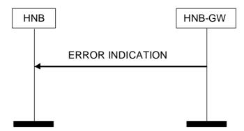
Figure 9 Error Indication HNB-GW Originated, Successful Operation
