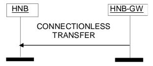
Figure 6: Connectionless Transfer to HNB
