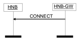
Figure 1A: Connect to HNB procedure
