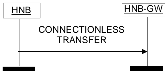
Figure 7: Connectionless Transfer to HNB-GW
