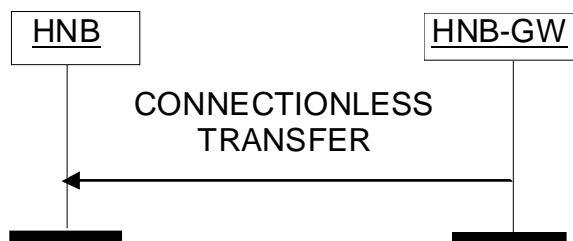
Figure 6: Connectionless Transfer to HNB
