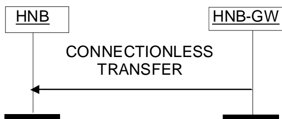
Figure 6: Connectionless Transfer to HNB
