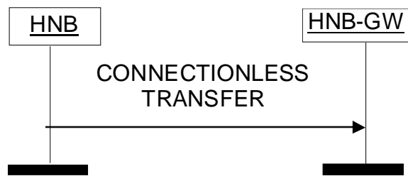
Figure 7: Connectionless Transfer to HNB-GW
