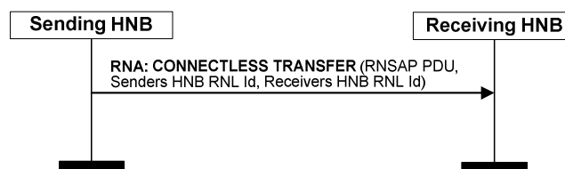
Figure 7.3.2.5.1-1: Connectionless data transfer – Direct Iurh-connectivity.
