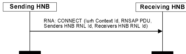
Figure 7.3.2.2.1-1: Signalling Connection Establishment – Direct Iurh-connectivity.
