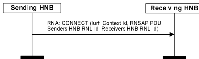
Figure 7.3.2.2.1-1: Signalling Connection Establishment – Direct Iurh-connectivity.
