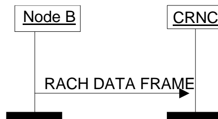
Figure 1: RACH Data Transfer procedure
