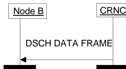
Figure 5: DSCH Data Transfer procedure
