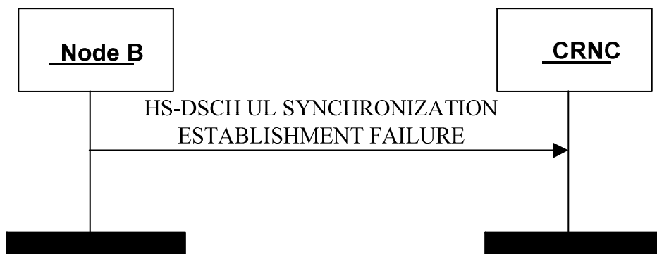
Figure 12D: HS-DSCH UL Synchronization Establishment Failure procedure
