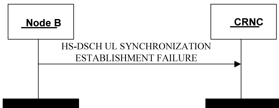
Figure 12D: HS-DSCH UL Synchronization Establishment Failure procedure
