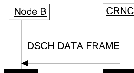
Figure 5: DSCH Data Transfer procedure
