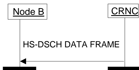
Figure 6A: HS-DSCH Data Transfer procedure
