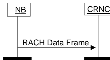
Figure 1: RACH Data Transfer Procedure
