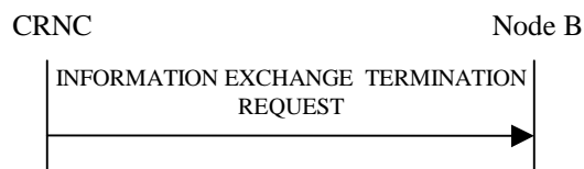
Figure 27O: Information Exchange Termination procedure, Successful Operation
