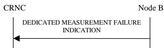
Figure 42: Dedicated Measurement Failure procedure, Successful Operation
