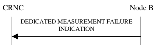
Figure 42: Dedicated Measurement Failure procedure, Successful Operation
