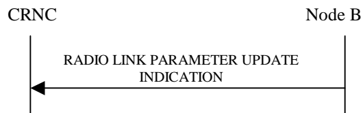
Figure 48: Radio Link Parameter Update Indication, Successful Operation
