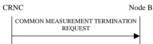
Figure 14: Common Measurement Termination procedure, Successful Operation
