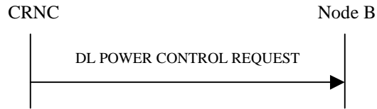
Figure 37: Downlink Power Control procedure, Successful Operation
