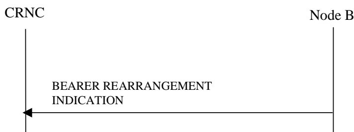
Figure 47C: Bearer Re-arrangement Indication, Successful Operation
