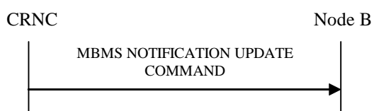
Figure 27Q: MBMS Notification Update procedure, Successful Operation
