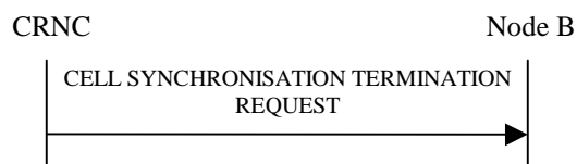
Figure 27H Cell Synchronisation Termination procedure, Successful Operation
