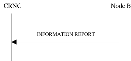
Figure 27N: Information Reporting procedure, Successful Operation
