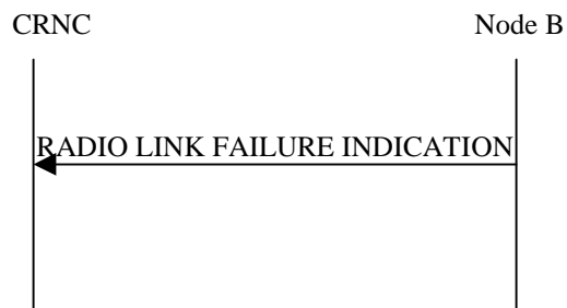
Figure 43: Radio Link Failure procedure, Successful Operation
