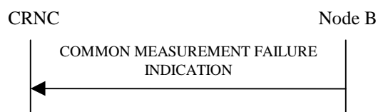
Figure 15: Common Measurement Failure procedure, Successful Operation
