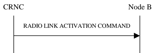
Figure 47D: Radio Link Activation procedure
