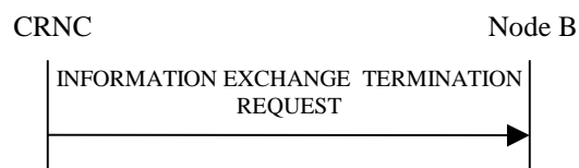
Figure 27O: Information Exchange Termination procedure, Successful Operation
