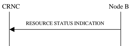
Figure 21: Resource Status Indication procedure, Successful Operation
