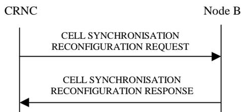
**Figure 27E Cell Synchronisation Reconfiguration procedure, Successful Operation**
