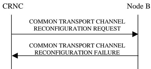
**Figure 4: Common Transport Channel Reconfiguration procedure, Unsuccessful Operation**
