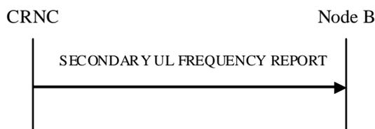
**Figure 48A: Secondary UL Frequency Reporting procedure**
