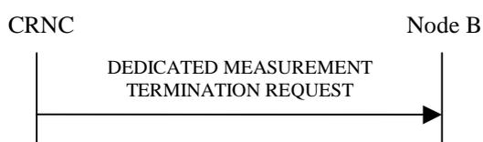
**Figure 41: Dedicated Measurement Termination procedure, Successful Operation**
