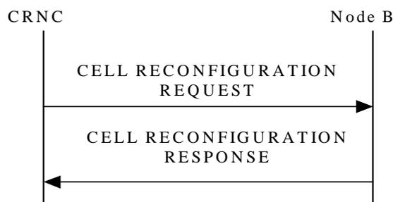
**Figure 18: Cell Reconfiguration procedure, Successful Operation**
