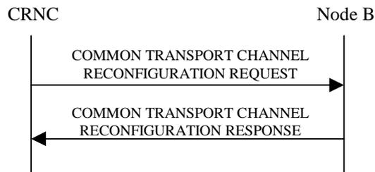
**Figure 3: Common Transport Channel Reconfiguration, Successful Operation**
