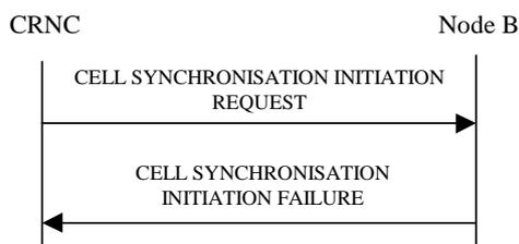
**Figure 27D Cell Synchronisation Initiation procedure, Unsuccessful Operation**
