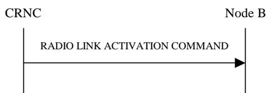
**Figure 47D: Radio Link Activation procedure**
