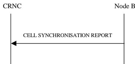
**Figure 27G Cell Synchronisation Reporting procedure, Successful Operation**
