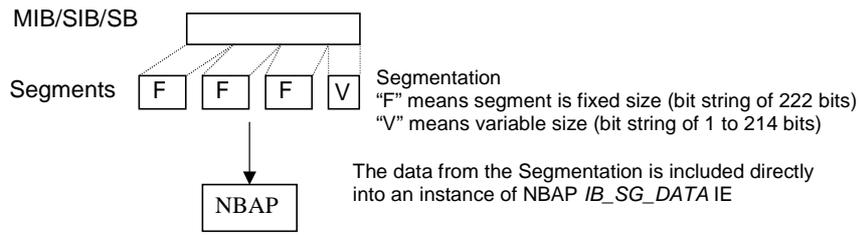
**Figure D.2: The Building of Segments**
