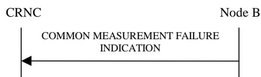
**Figure 15: Common Measurement Failure procedure, Successful Operation**
