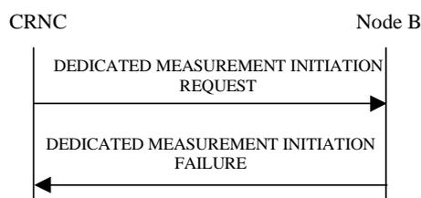
Figure 39: Dedicated Measurement Initiation procedure: Unsuccessful Operation
