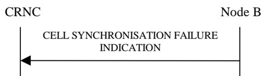
**Figure 271 Cell Synchronisation Failure procedure, Successful Operation**
