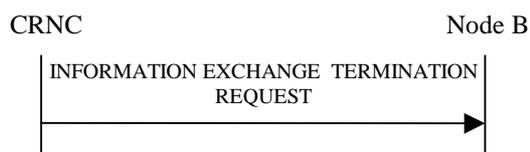
**Figure 27O: Information Exchange Termination procedure, Successful Operation**
