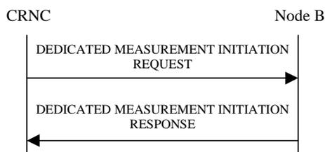
**Figure 38: Dedicated Measurement Initiation procedure, Successful Operation**
