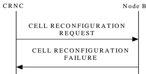
**Figure 19: Cell Reconfiguration procedure: Unsuccessful Operation**
