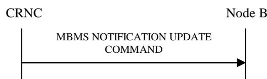
**Figure 27Q: MBMS Notification Update procedure, Successful Operation**
