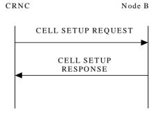
Figure 16: Cell Setup procedure, Successful Operation
