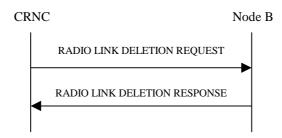
Figure 36: Radio Link Deletion procedure, Successful Operation
