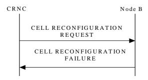
Figure 19: Cell Reconfiguration procedure: Unsuccessful Operation
