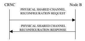
Figure 26: Physical Shared Channel Reconfiguration, Successful Operation
