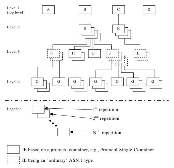
Figure C.1: Example of content of a received NBAP message based on the EXAMPLE MESSAGE
