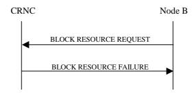
Figure 7: Block Resource procedure, Unsuccessful Operation
