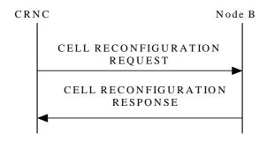
Figure 18: Cell Reconfiguration procedure, Successful Operation
