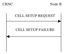
Figure 17: Cell Setup procedure: Unsuccessful Operation
