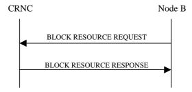
Figure 6: Block Resource procedure, Successful Operation
