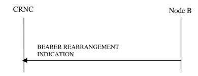
Figure 47C: Bearer Re-arrangement Indication, Successful Operation
