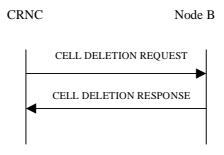
Figure 20: Cell Deletion procedure, Successful Operation
