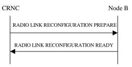
Figure 30: Synchronised Radio Link Reconfiguration Preparation procedure, Successful Operation
