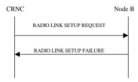
Figure 25: Radio Link Setup procedure, Unsuccessful Operation
