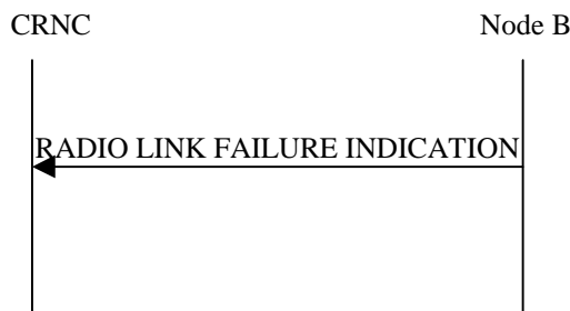
Figure 43: Radio Link Failure procedure, Successful Operation
