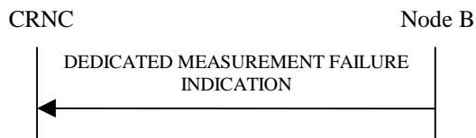
Figure 42: Dedicated Measurement Failure procedure, Successful Operation
