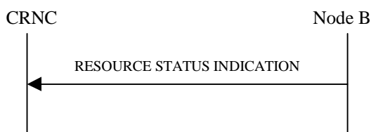
Figure 21: Resource Status Indication procedure, Successful Operation
