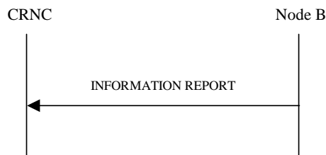
Figure 27N: Information Reporting procedure, Successful Operation
