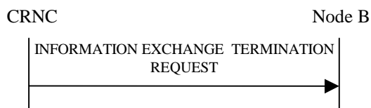
Figure 27O: Information Exchange Termination procedure, Successful Operation
