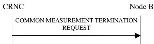
Figure 14: Common Measurement Termination procedure, Successful Operation
