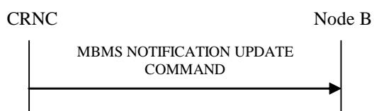
Figure 27Q: MBMS Notification Update procedure, Successful Operation
