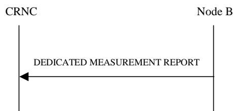
Figure 40: Dedicated Measurement Reporting procedure, Successful Operation
