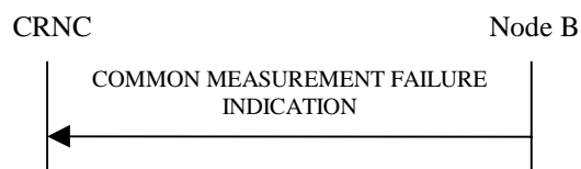
Figure 15: Common Measurement Failure procedure, Successful Operation
