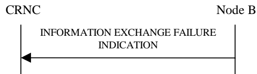
Figure 27P: Information Exchange Failure procedure, Successful Operation
