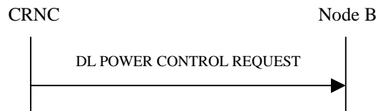
Figure 37: Downlink Power Control procedure, Successful Operation
