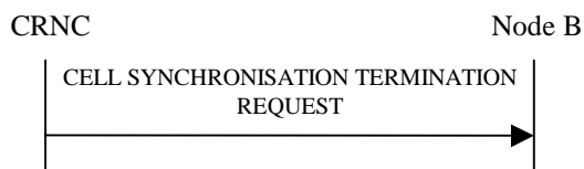
Figure 27H Cell Synchronisation Termination procedure, Successful Operation
