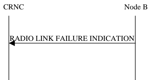
Figure 43: Radio Link Failure procedure, Successful Operation
