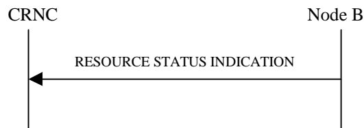
Figure 21: Resource Status Indication procedure, Successful Operation
