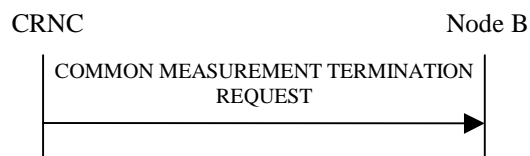
Figure 14: Common Measurement Termination procedure, Successful Operation
