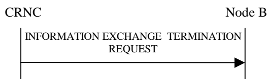
Figure 27O: Information Exchange Termination procedure, Successful Operation
