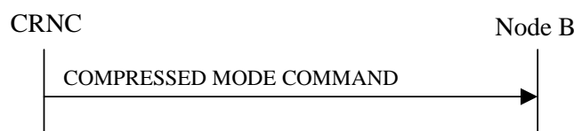
Figure 47: Compressed Mode Command procedure, Successful Operation
