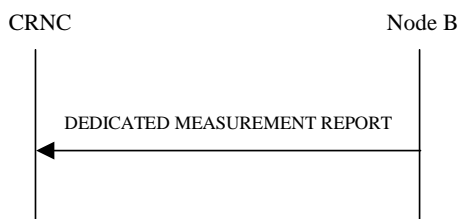
Figure 40: Dedicated Measurement Reporting procedure, Successful Operation
