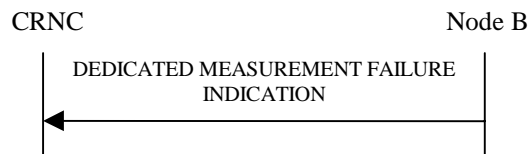
Figure 42: Dedicated Measurement Failure procedure, Successful Operation
