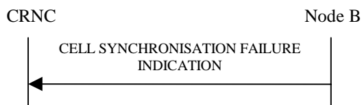
Figure 27I Cell Synchronisation Failure procedure, Successful Operation
