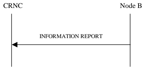
Figure 27N: Information Reporting procedure, Successful Operation
