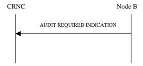
Figure 9: Audit Required procedure, Successful Operation
