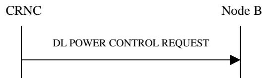
Figure 37: Downlink Power Control procedure, Successful Operation
