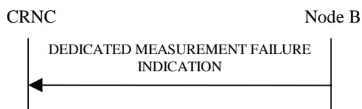
Figure 42: Dedicated Measurement Failure procedure, Successful Operation
