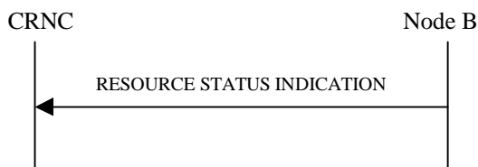
Figure 21: Resource Status Indication procedure, Successful Operation
