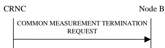
Figure 14: Common Measurement Termination procedure, Successful Operation
