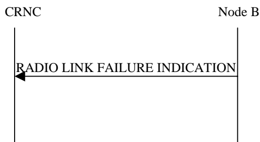
Figure 43: Radio Link Failure procedure, Successful Operation
