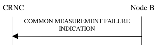
Figure 15: Common Measurement Failure procedure, Successful Operation
