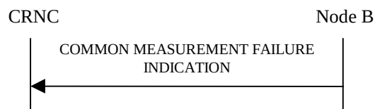
Figure 15: Common Measurement Failure procedure, Successful Operation
