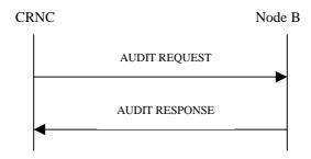
Figure 10: Audit procedure, Successful Operation
