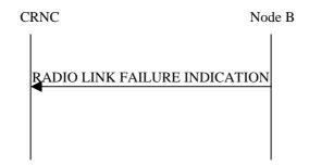
Figure 43: Radio Link Failure procedure, Successful Operation
