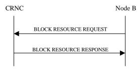
Figure 6: Block Resource procedure, Successful Operation
