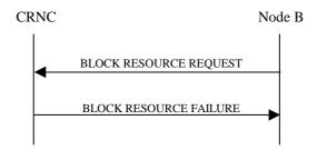
Figure 7: Block Resource procedure, Unsuccessful Operation
