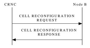
Figure 18: Cell Reconfiguration procedure, Successful Operation
