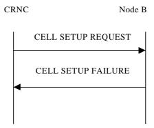
Figure 17: Cell Setup procedure: Unsuccessful Operation
