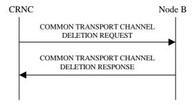
Figure 5: Common Transport Channel Deletion procedure, Successful Operation
