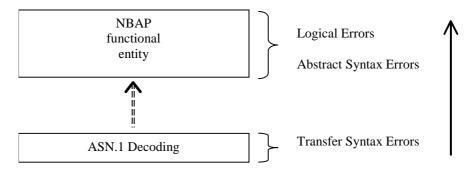
Figure 38: Protocol Errors in NBAP.
