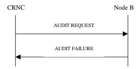
Figure 10A: Audit procedure, Unsuccessful Operation
