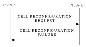
Figure 19: Cell Reconfiguration procedure: Unsuccessful Operation
