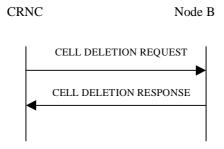
Figure 20: Cell Deletion procedure, Successful Operation
