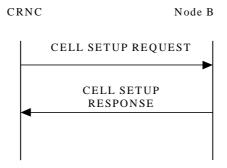
Figure 16: Cell Setup procedure, Successful Operation
