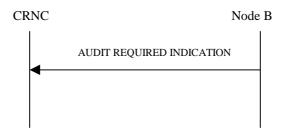
Figure 9: Audit Required procedure, Successful Operation
