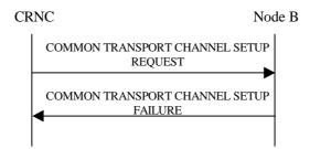
Figure 2: Common Transport Channel Setup procedure, Unsuccessful Operation
