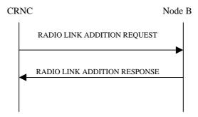
Figure: 28 Radio Link Addition procedure, Successful Operation
