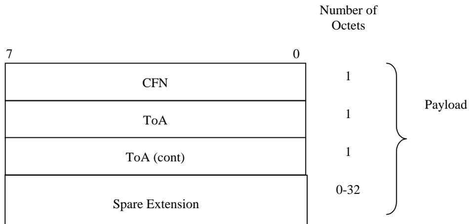
**Figure 16: Structure of the UL Synchronisation control frame**
