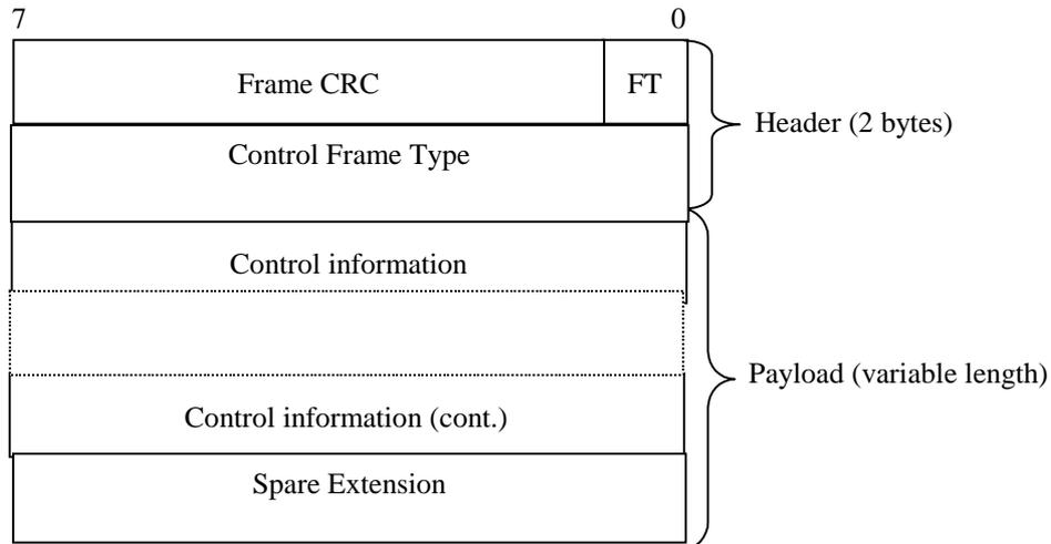
**Figure 13: General structure of the control frames**
