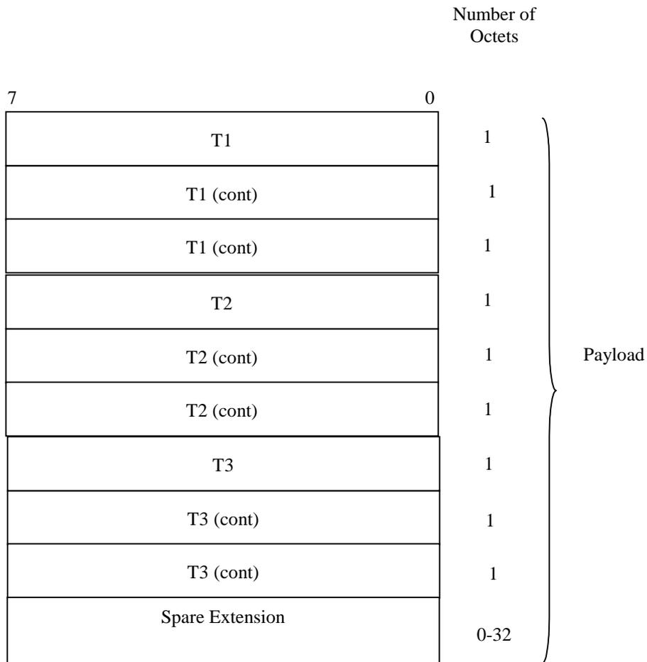
**Figure 19: Structure of the payload for UL Node Synchronisation control frame**
