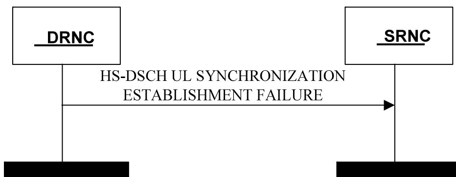
Figure 4AC: HS-DSCH UL Synchronization Establishment Failure procedure
