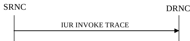
Figure 26K: Iur Invoke Trace procedure, Successful Operation
