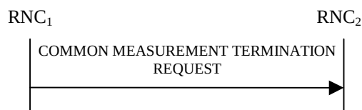
Figure 30D: Common Measurement Termination procedure, Successful Operation
