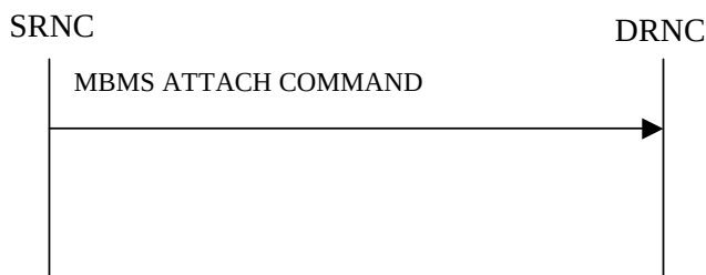
Figure 31: MBMS Attach procedure, Successful Operation
