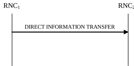
Figure 30L: Direct Information Transfer procedure, Successful Operation
