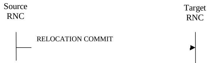
Figure 3: Relocation Commit procedure, Successful Operation
