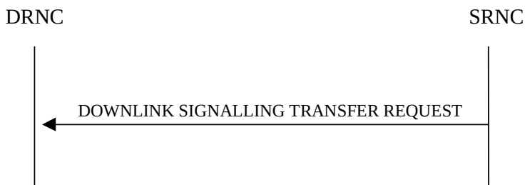
Figure 2: Downlink Signalling Transfer procedure, Successful Operation
