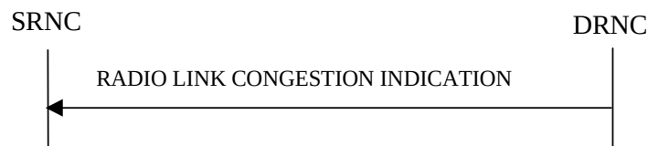
Figure 26C: Radio Link Congestion procedure, Successful Operation
