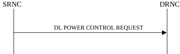
Figure 25: Downlink Power Control procedure, Successful Operation
