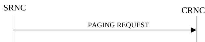
Figure 4: Paging procedure, Successful Operation
