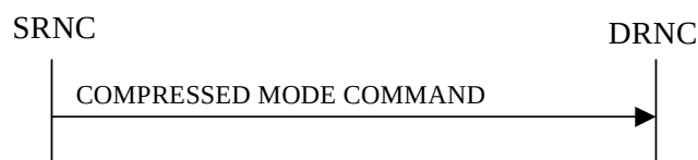
Figure 26: Compressed Mode Command procedure, Successful Operation
