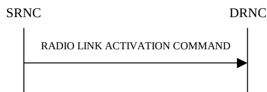
Figure 26D: Radio Link Activation procedure
