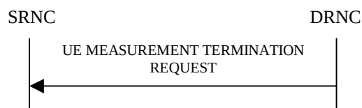
Figure 26I: UE Measurement Termination procedure, Successful Operation
