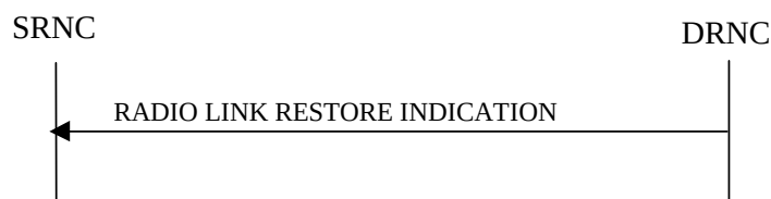
Figure 19: Radio Link Restoration procedure, Successful Operation
