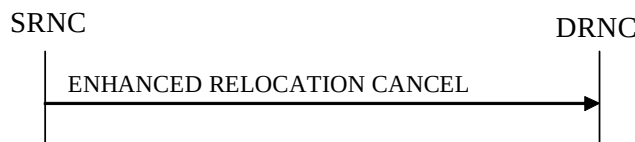
Figure 26O: Enhanced Relocation Cancel procedure: Successful Operation
