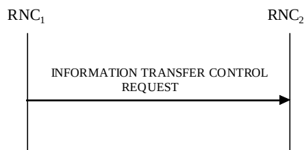
Figure 30M: Information Transfer Control procedure, Successful Operation
