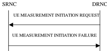
**Figure 26G: UE Measurement Initiation procedure, Unsuccessful Operation**
