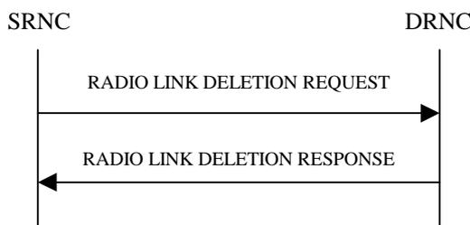
**Figure 9: Radio Link Deletion procedure, Successful Operation**
