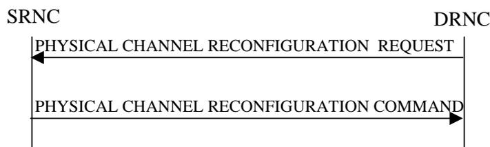
**Figure 16: Physical Channel Reconfiguration procedure, Successful Operation**
