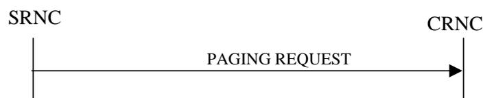
**Figure 4: Paging procedure, Successful Operation**
