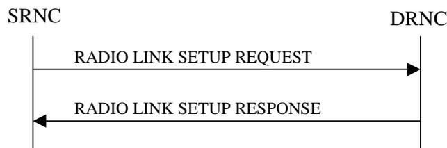
**Figure 5: Radio Link Setup procedure: Successful Operation**
