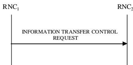
**Figure 30M: Information Transfer Control procedure, Successful Operation**
