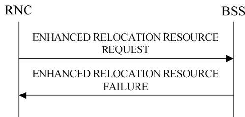
**Figure 4C: Enhanced Relocation Resource Allocation Procedure, Unsuccessful Operation**
