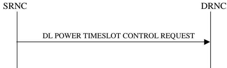
**Figure 26A: Downlink Power Timeslot Control procedure, Successful Operation**
