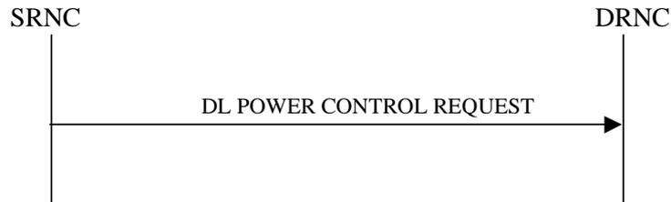
**Figure 25: Downlink Power Control procedure, Successful Operation**
