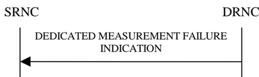
**Figure 24: Dedicated Measurement Failure procedure, Successful Operation**
