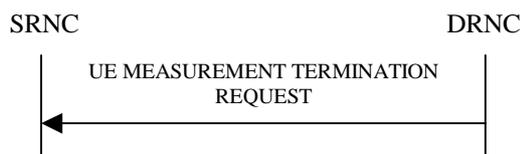
**Figure 26I: UE Measurement Termination procedure, Successful Operation**
