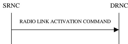
**Figure 26D: Radio Link Activation procedure**
