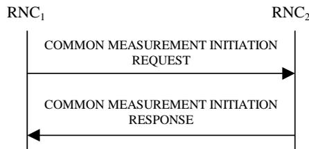
**Figure 30A: Common Measurement Initiation procedure, Successful Operation**
