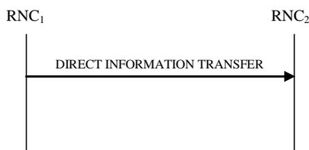
**Figure 30L: Direct Information Transfer procedure, Successful Operation**
