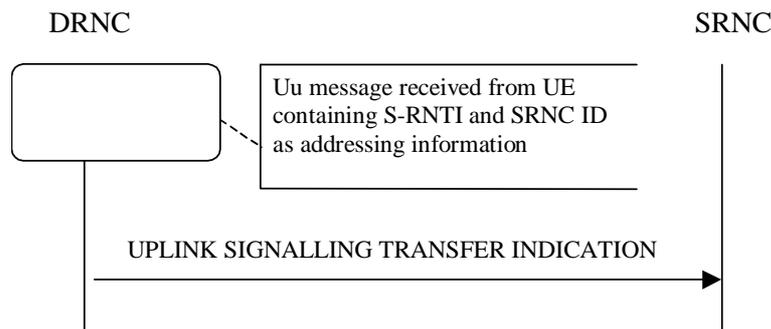
**Figure 1: Uplink Signalling Transfer procedure, Successful Operation**
