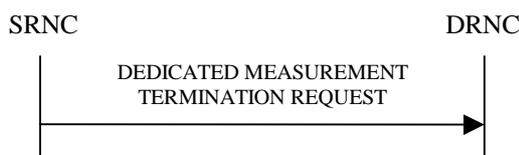
**Figure 23: Dedicated Measurement Termination procedure, Successful Operation**
