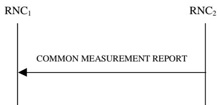
**Figure 30C: Common Measurement Reporting procedure, Successful Operation**
