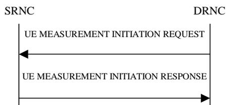
Figure 26F: UE Measurement Initiation procedure, Successful Operation
