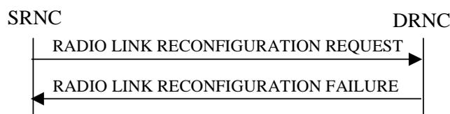
**Figure 15: Unsyncronised Radio Link Reconfiguration procedure, Unsuccessful Operation**
