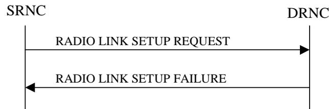
**Figure 6: Radio Link Setup procedure: Unsuccessful Operation**
