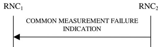
**Figure 30E: Common Measurement Failure procedure, Successful Operation**
