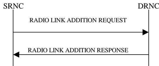
**Figure 7: Radio Link Addition procedure: Successful Operation**
