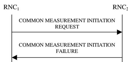
Figure 30B: Common Measurement Initiation procedure, Unsuccessful Operation
