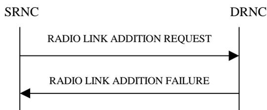
**Figure 8: Radio Link Addition procedure: Unsuccessful Operation**
