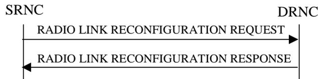
**Figure 14: Unsynchronised Radio Link Reconfiguration procedure, Successful Operation**
