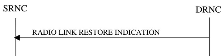
**Figure 19: Radio Link Restoration procedure, Successful Operation**
