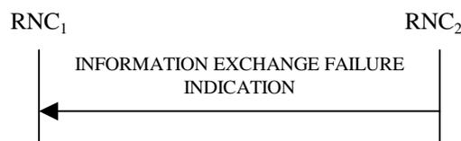
**Figure 30J: Information Exchange Failure procedure, Successful Operation**
