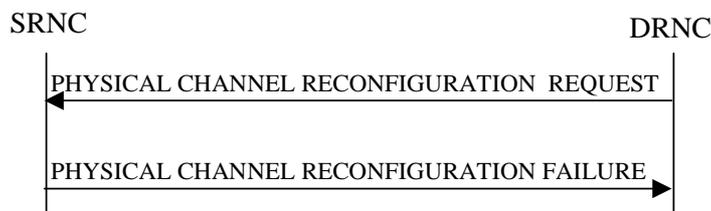
**Figure 17: Physical Channel Reconfiguration procedure, Unsuccessful Operation**
