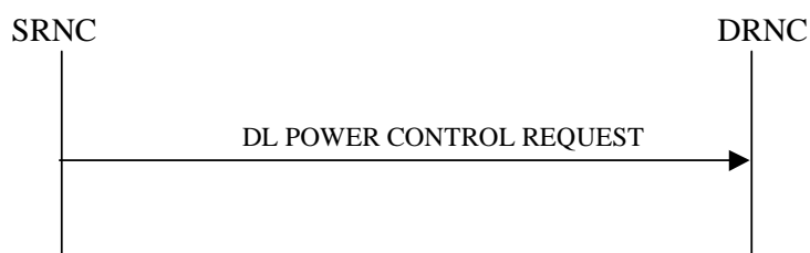
Figure 25: Downlink Power Control procedure, Successful Operation
