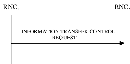
Figure 30M: Information Transfer Control procedure, Successful Operation
