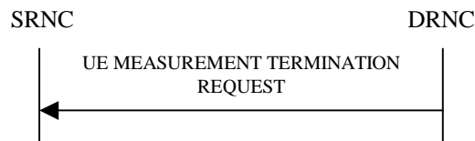
Figure 26I: UE Measurement Termination procedure, Successful Operation
