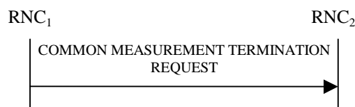
Figure 30D: Common Measurement Termination procedure, Successful Operation
