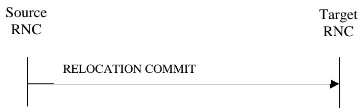
Figure 3: Relocation Commit procedure, Successful Operation
