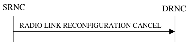
Figure 13: Synchronised Radio Link Reconfiguration Cancellation procedure, Successful Operation
