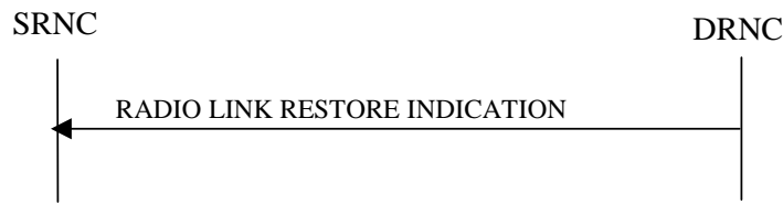
Figure 19: Radio Link Restoration procedure, Successful Operation
