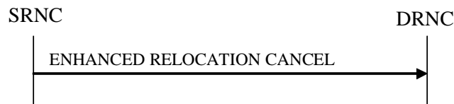
Figure 26O: Enhanced Relocation Cancel procedure: Successful Operation
