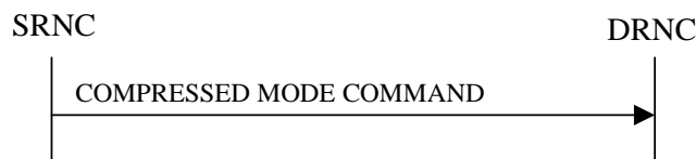
Figure 26: Compressed Mode Command procedure, Successful Operation
