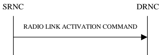
Figure 26D: Radio Link Activation procedure
