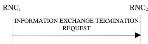
Figure 30I: Information Exchange Termination procedure, Successful Operation
