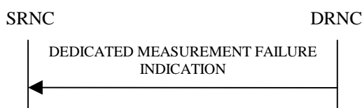
Figure 24: Dedicated Measurement Failure procedure, Successful Operation
