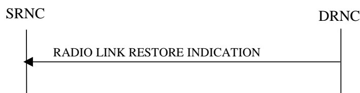
Figure 19: Radio Link Restoration procedure, Successful Operation
