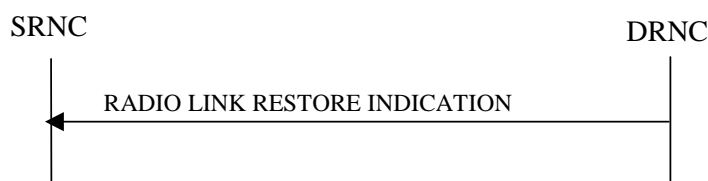
Figure 19: Radio Link Restoration procedure, Successful Operation
