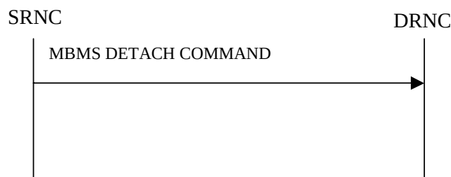
Figure 32: MBMS Detach procedure, Successful Operation
