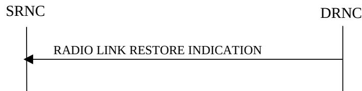
Figure 19: Radio Link Restoration procedure, Successful Operation
