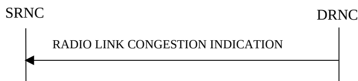
Figure 26C: Radio Link Congestion procedure, Successful Operation
