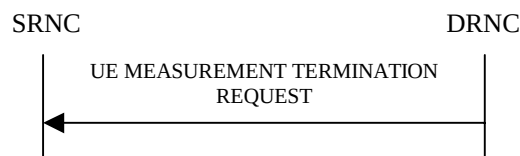
Figure 26I: UE Measurement Termination procedure, Successful Operation
