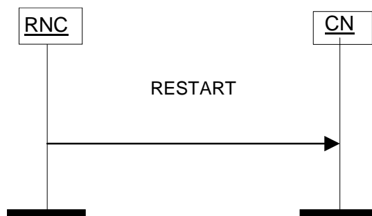
Figure 11: Restart Indication Procedure: Successful Operation
