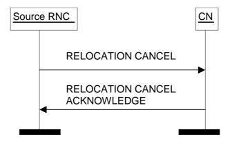
Figure 11: Relocation Cancel procedure. Successful operation.
