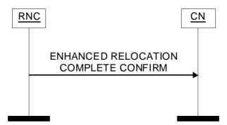
Figure 70: Enhanced Relocation Complete Confirm procedure. Successful operation.
