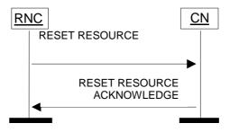
Figure 34: RNC initiated Reset Resource procedure. Successful operation.
