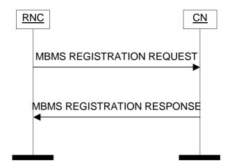
Figure 52: MBMS Registration procedure. Successful operation.
