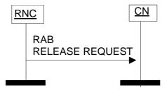
Figure 2: RAB Release Request procedure. Successful operation.
