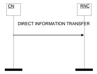
Figure 43: Information Request procedure. Successful operation.
