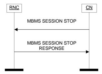
Figure 50: MBMS Session Stop procedure. Successful operation.
