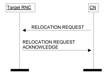
Figure 7: Relocation Resource Allocation procedure. Successful operation.
