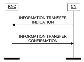
Figure 39: Information Transfer procedure. Successful operation.
