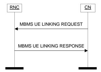
Figure 51: MBMS UE Linking procedure. Successful operation.
