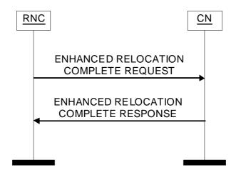
Figure 58: Enhanced Relocation Complete procedure. Successful operation.
