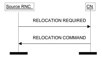
Figure 5: Relocation Preparation procedure. Successful operation.
