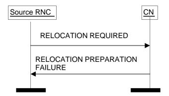
Figure 6: Relocation Preparation procedure. Unsuccessful operation.
