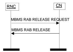
Figure 56: MBMS RAB Release procedure. Successful operation.
