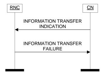
Figure 40: Information Transfer procedure. Unsuccessful operation.
