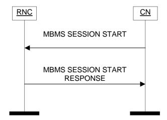
Figure 46: MBMS Session Start procedure. Successful operation.
