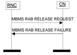
Figure 57: MBMS RAB RELEASE procedure. Unsuccessful operation.
