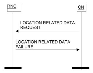
Figure 38: Location Related Data procedure. Unsuccessful operation.
