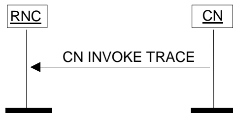
Figure 18: CN Invoke Trace procedure. Successful operation.
