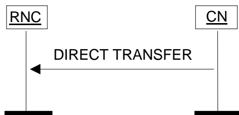
Figure 25: Direct Transfer, CN originated. Successful operation.
