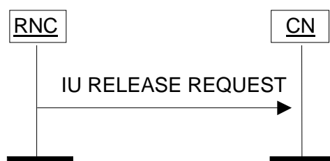
Figure 3: Iu Release Request procedure. Successful operation.
