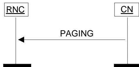
Figure 16: Paging procedure. Successful operation.
