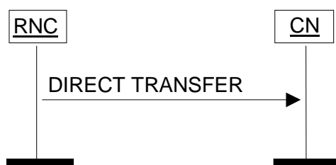
Figure 26: Direct Transfer, RNC originated. Successful operation.
