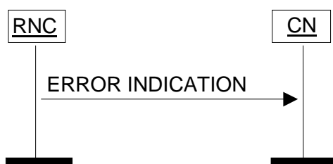
Figure 32: Error Indication procedure, RNC originated. Successful operation.
