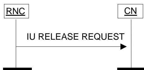
Figure 3: Iu Release Request procedure. Successful operation.
