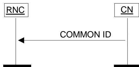
Figure 17: Common ID procedure. Successful operation.
