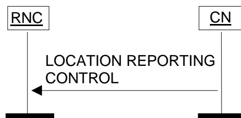
Figure 21: Location Reporting Control procedure. Successful operation.
