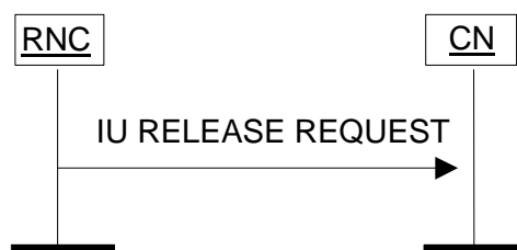
Figure 3: Iu Release Request procedure. Successful operation.
