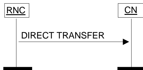
Figure 26: Direct Transfer, RNC originated. Successful operation.
