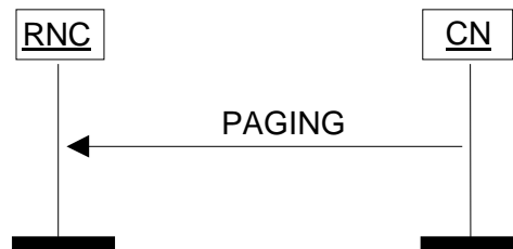
Figure 16: Paging procedure. Successful operation.
