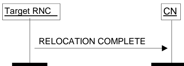
Figure 10: Relocation Complete procedure. Successful operation.
