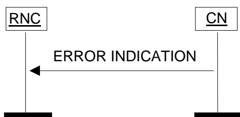
Figure 31: Error Indication procedure, CN originated. Successful operation.
