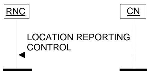
Figure 21: Location Reporting Control procedure. Successful operation.
