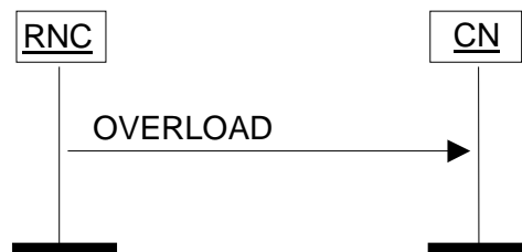
Figure 28: Overload at the UTRAN. Successful operation.
