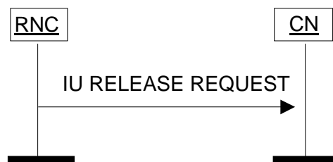
Figure 3: Iu Release Request procedure. Successful operation.
