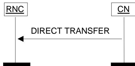
Figure 25: Direct Transfer, CN originated. Successful operation.
